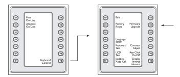
Figure 3 – IntuiKey Keyboard Bootloader Menu Access
